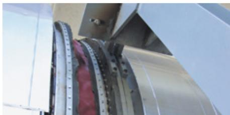
**DRO** Rotary kiln sealing system in a plant for incinerating chemical residues at Infracor GmbH at the Chemiepark in Marl, Germany.
