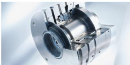
In an air separation plant in Austria, the compressor for production of technical gases is sealed by a gas-lubricated **DGS20** mechanical seal. Operating conditions:  $p = 7 \dots 30 \text{ bar}$  (102 ... 435 PSI);  $t = 40 \dots 70 \text{ °C}$  (104 ... 158 °F);  $n = 10,000 \dots 20,250 \text{ min}^{-1}$ .
