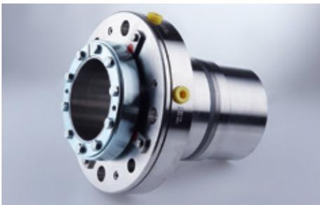
During the production of ammonia, carbon dioxide is removed from the process with Benfield solution – an aqueous potassium carbonate solution with diethanolamine. **HJS1** type mechanical seals have proven to be best for sealing the pumps in this area. Typical operating conditions:  $p = 2 \dots 4 \text{ bar}$  (29 ... 58 PSI);  $t = 100 \dots 150 \text{ }^\circ\text{C}$  (212 ... 302  $^\circ\text{F}$ );  $n = 1,500 \text{ min}^{-1}$ .
