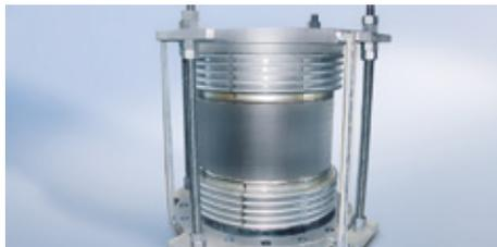
**Expansion joints** are used in pipes carrying steam at Eastman Chemical Co. in Kingsport, USA. Operating conditions:  $p = 0.55\text{ bar}$  (8 PSI);  $t = 427\text{ }^{\circ}\text{C}$  ( $800\text{ }^{\circ}\text{F}$ ).
