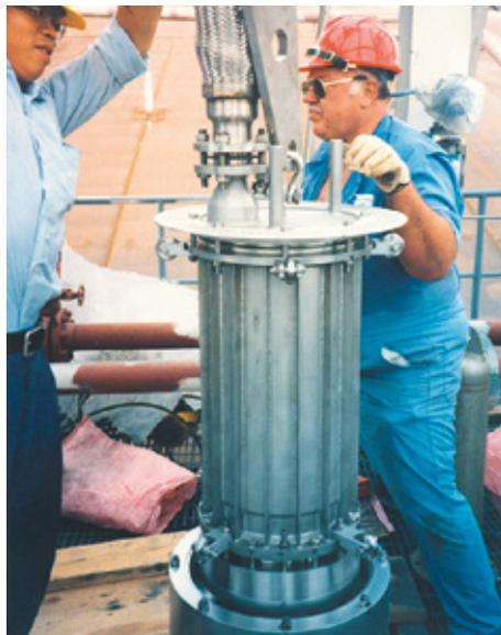
The high-efficiency **NMB-16P-2R-45-SC** magnetic coupling as a hermetic seal in a vertical pump. The process medium – a mixture of ammonia and propane – has very poor lubricating properties. The low temperature ( $-45 \text{ }^\circ\text{C}$  ( $-49 \text{ }^\circ\text{F}$ )) plays a decisive role in the choice of materials.
